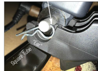
Arrow Shows “Ear” Stopping on Motor Pin
